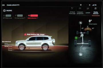
Wading Depth Detection Water depth detection system
