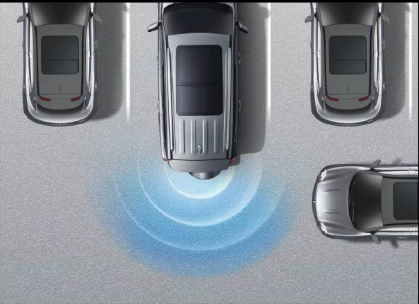
RCTA REAR CROSS TRAFFIC ALERT RCTB REAR CROSS TRAFFIC BRAKING
