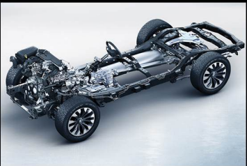
Professional off-road suspension and body-on-frame chassis
